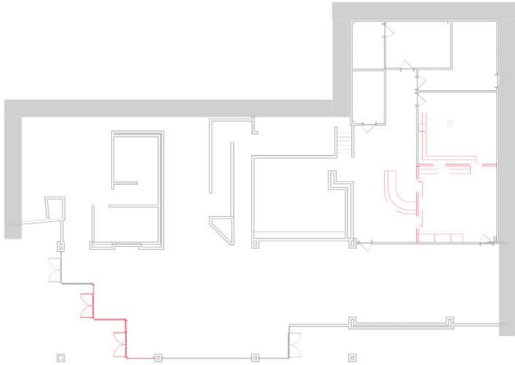
DEMOLITION PLAN *RED LINES INDICATE DEMO
